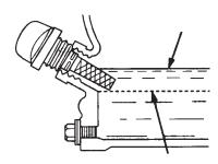
Figure 9. Engine Oil Dipstick (Oil Level)
